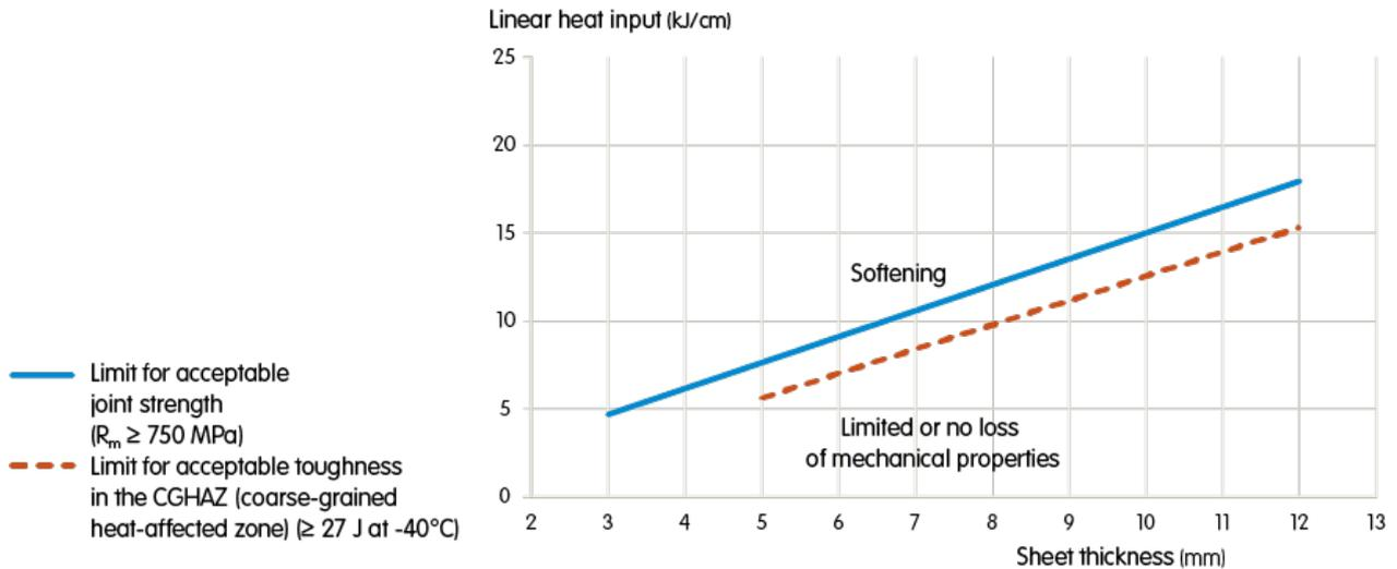
Recommendations for selecting the suitable heat input for MAG welding of Armstrong® Ultra 700MC grade.
